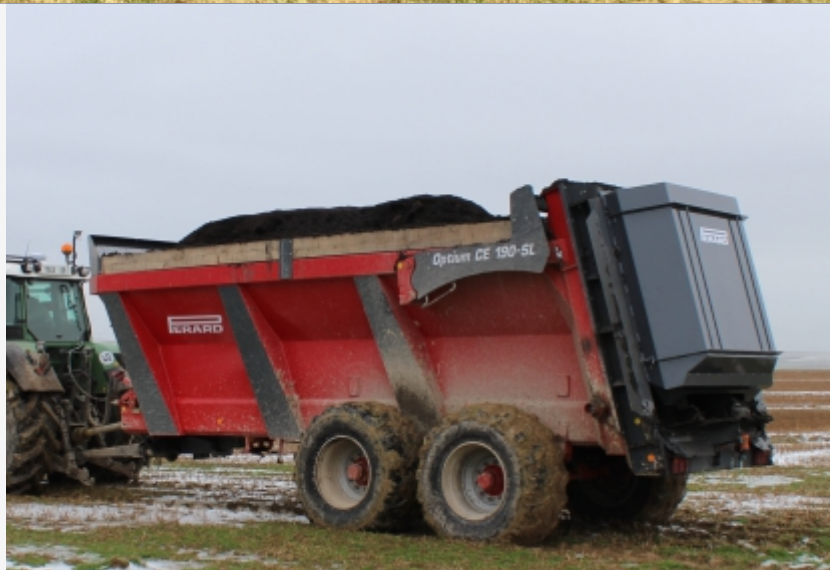
Rotors covering for dry compost
