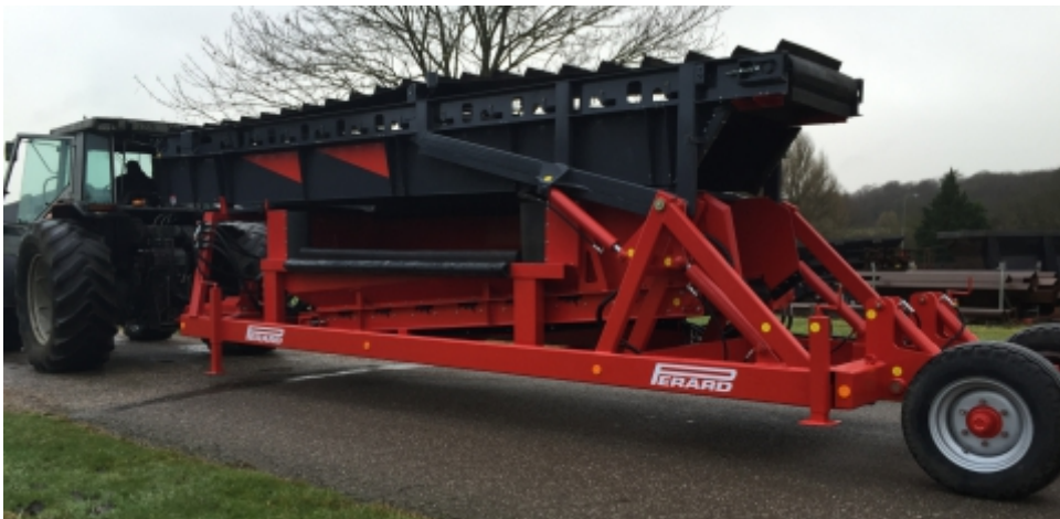
General drive by the hydraulic unit driven by the power take-off – Power required: 80 HP minimum
