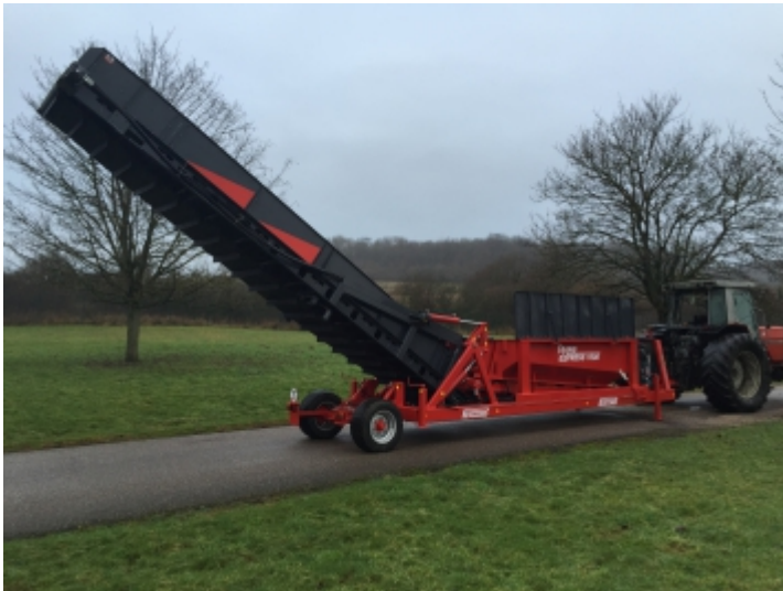
General drive by the hydraulic unit driven by the power take-off – Power required: 80 HP minimum
