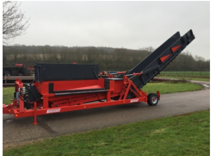
General drive by the hydraulic unit driven by the power take-off – Power required: 80 HP minimum
