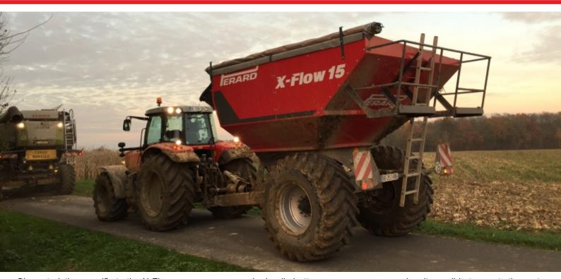
Characteristics specific to the X-Flow (except 15 and 19): a hydraulic bottom screw conveyor makes it possible to empty the cart completely and obtain the same discharge rate from start to finish. The 3.50m axle track width means that the cart does not follow in the tractor's track and provides exceptional stability.
