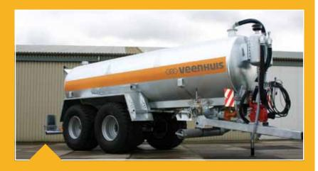
These tankers can be equipped with various options, such as a suction arm, an internal mixing system, or an unloading arm for quick unloading.
