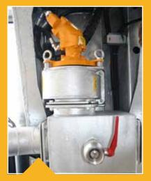
Because of the header tank with loading turbo underneath the tanker, the loading turbo can be used with both left and right valves (or possibly a suction arm) to ensure the shortest waiting time.
