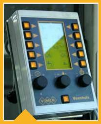
The Ecoline is available with a Premium CAN-bus controlsystem, for easy control of the tanker.
