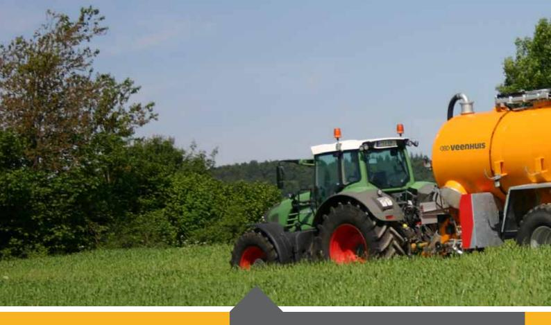
The Ecoline tankers are available with a single-acting hitch for draghose systems or trailing shoe injectors
