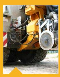
The double-acting hitch is high quality, and can couple different injectors.
