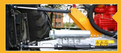
The tractor has optimal traction because of the suspended drawbar in combination with a toplink cylinder.
